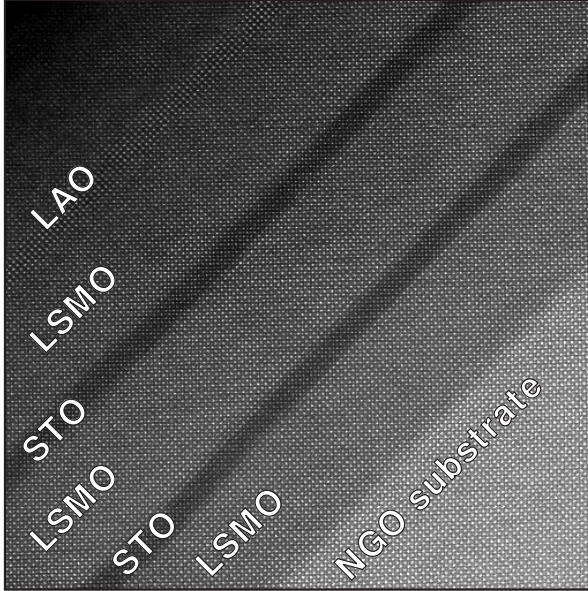
Figure 1.1: An example of a perovskite oxide multilayer structure with layers of \text{La}_{0.67}\text{Sr}_{0.33}\text{MnO}_3 (LSMO), \text{SrTiO}_3 (STO) and \text{LaAlO}_3 (LAO) grown on a \text{NdGaO}_3 (NGO) substrate. This image was measured at Chalmers University of Technology, Sweden.
